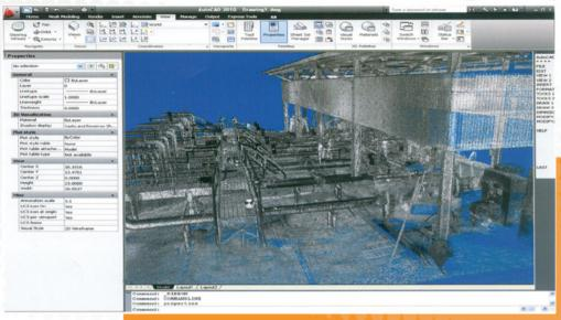
RSG Inc. can support your plant relocation project using 3D Laser Scanning to accurately document both the physical plant layout and individual assets.
